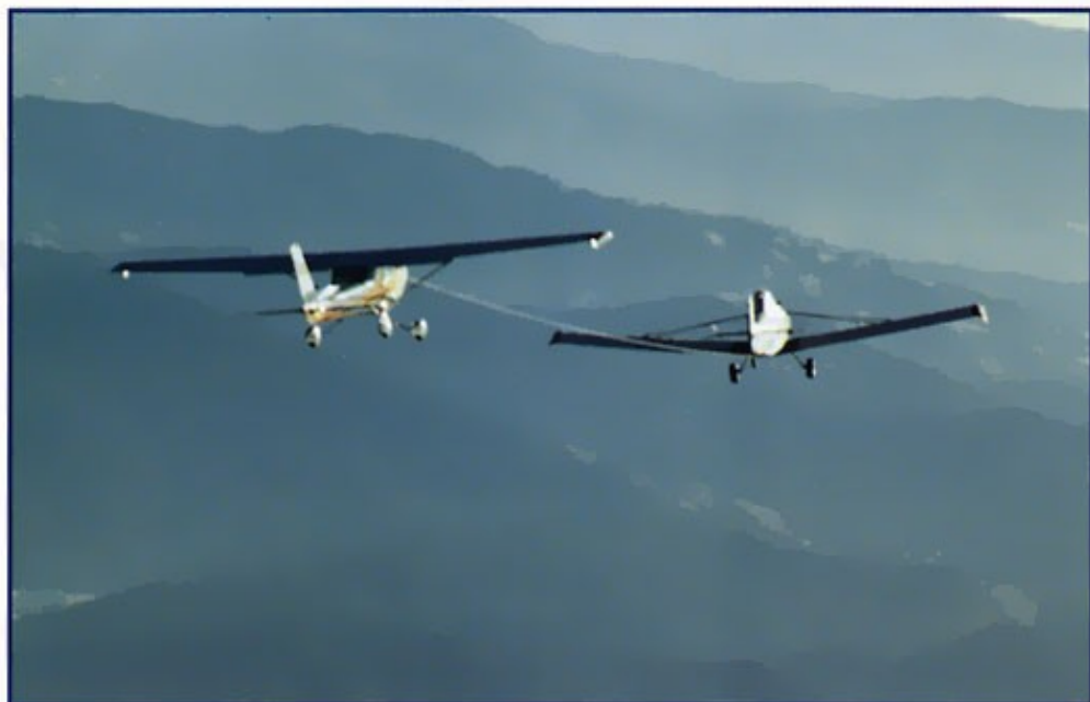
CAFE Foundation Chief Test Pilot, C.J. Stephens, in the propless Cessna 152 as it is towed aloft by the Piper Pawnee over California's Mendocino Coast. The Cessna's glide ratio is approximately 13 to 1.
