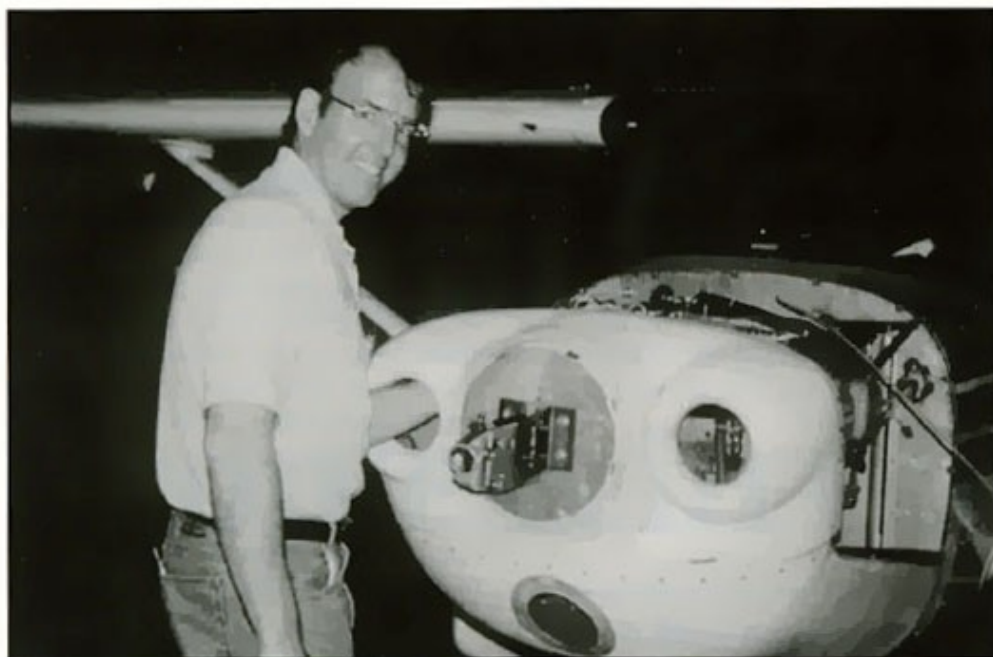
Brien Seeley installs the Tost tow hook onto the Cessna crankshaft flange.
